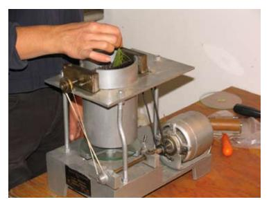
**Figure 4.3** - This piece of equipment is used in counting spider mites. Fine brushes remove mites from foliage where they fall onto a plate. Individuals on the plate are counted. The brushes are thorough, so the counts are very accurate as long as the foliage is collected in such a way that reduces undersampling and sampling bias.
