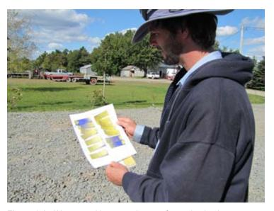
**Figure 6.1** - Water sensitive paper is great for evaluating how your sprayer works in the field. By setting pieces of water sensitive paper in different places among the plants you spray, you can see where your spraying equipment is successful.
