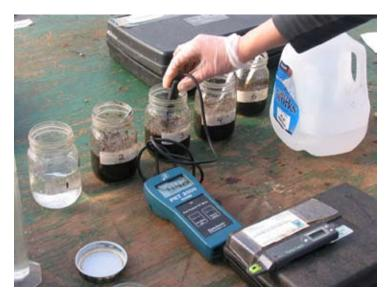
**Figure 1.1** - This pictures shows a pest manager testing electrical conductivity (EC) in container production. The EC of a medium is directly related to the concentration of ions it holds, so a higher EC reading means there are more ions in the medium. Since plants can only take up ions, a higher EC means there are more elements available to the plant.
