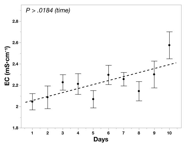
**Figure 1.** Electrical conductivity of a bark-based substrate over time following incorporation of a controlled-release fertilizer.
